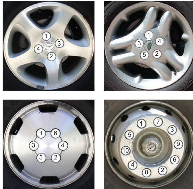
Figure 4.141 Torque sequences
